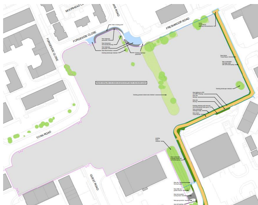
Figure 2: Proposed site layout with active travel route shown in yellow, pavement highway works to the north and the turning head to the south.
