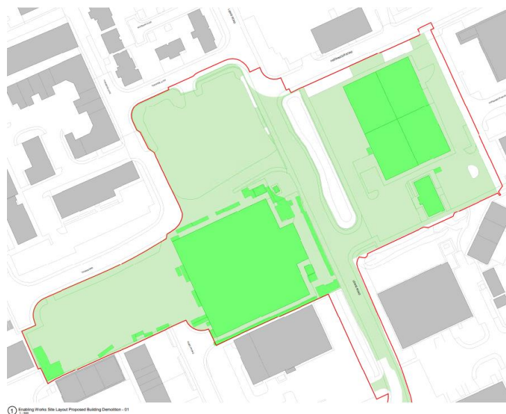
Figure 4: The bright green shading shows the buildings that will be demolished and the lighter shade of green shows the hardstanding and vegetation to be removed.
